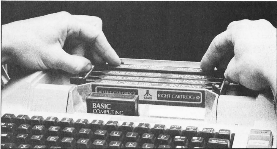
FIGURE 2-17. Removing a RAM memory module (ATARI 800 computer only)
