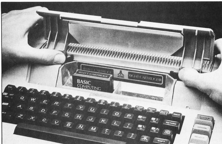
FIGURE 2-15. Releasing the ATARI 800 computer top cover latches
