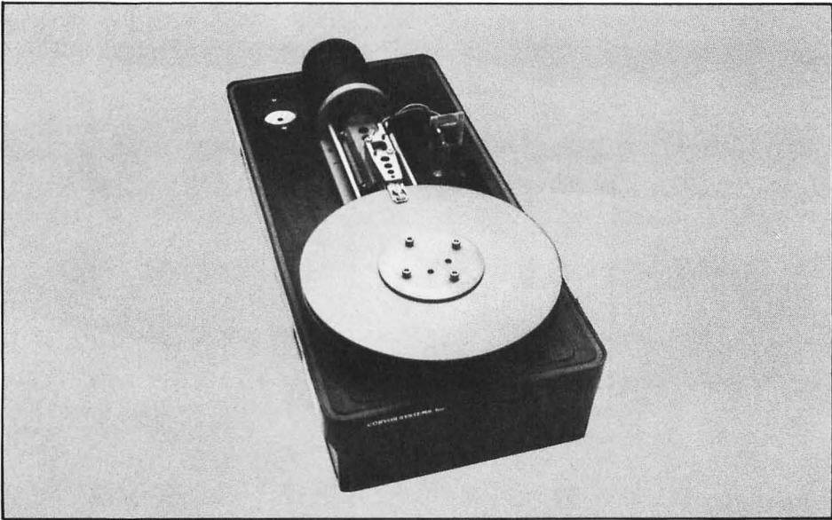
FIGURE 7-2. Winchester disk drive (Shown with cover removed)
